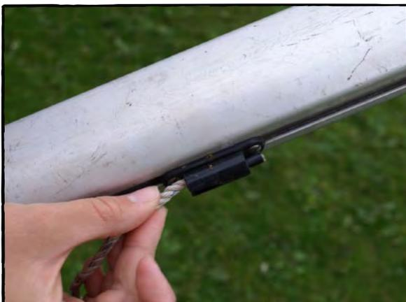
Photo 17, Feed the outhaul rope through the cleat
