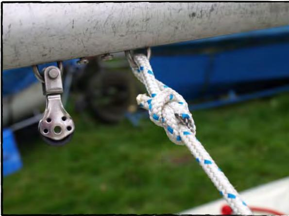
Photo 32, Attach main sheet to the boom
