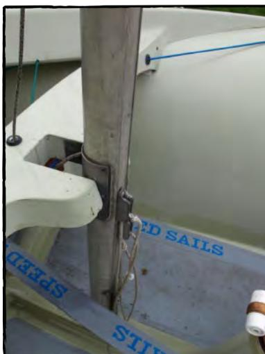
Photo 2, mast and jammers
