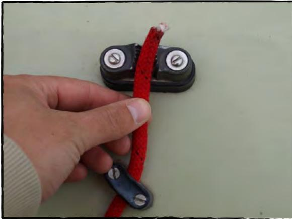
Photo 13, Pass the jib sheets through the jammers
