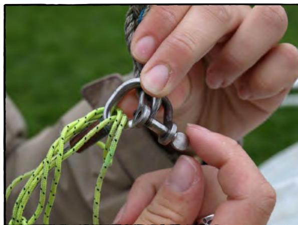
Photo 9, Attach the jib to the halyard
