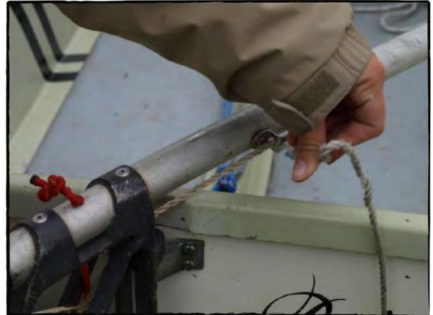
Photo 37, Attach the rudder uphaul
