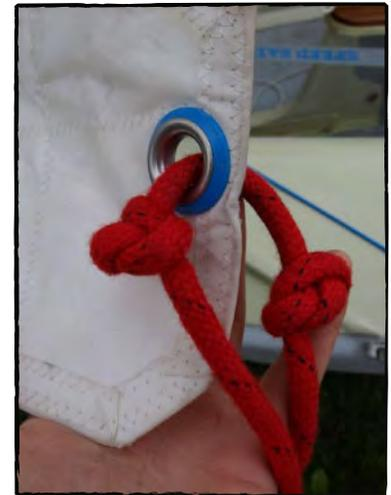
Photo 12, attach the jib sheet
