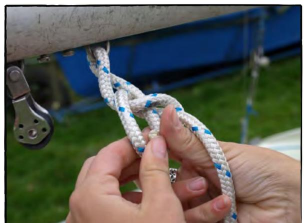
Photo 31, attach the mainsheet to the boom
