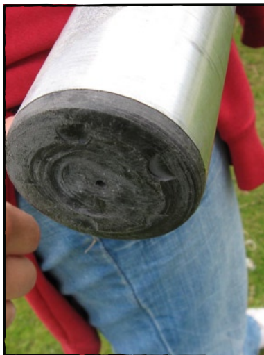
Photo 10, Clean the mast foot
