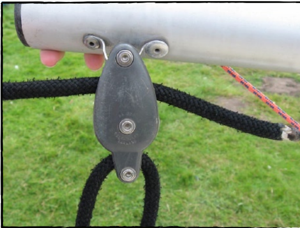
Photo 33, Back through first block
