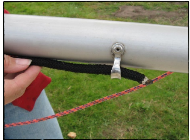
Photo 34, Through eyehole on boom
