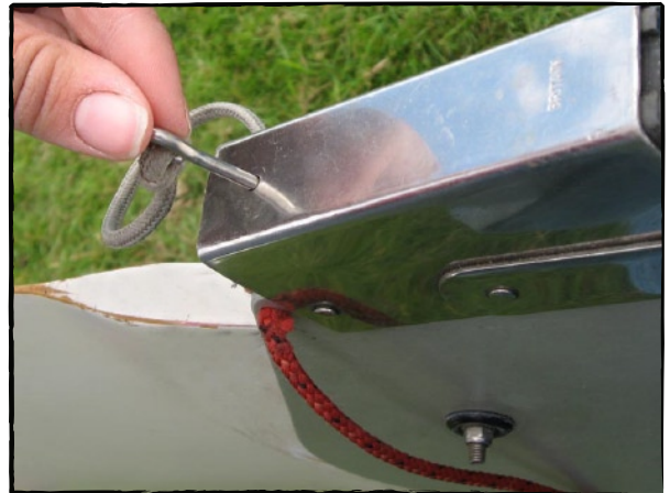
Photo 39, Secure the tiller
