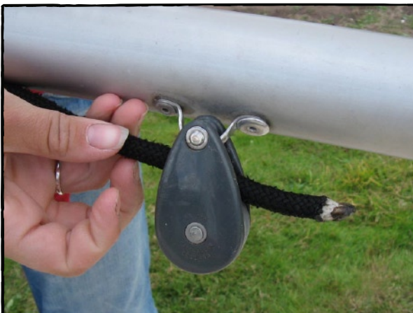
Photo 35, Through block on boom
