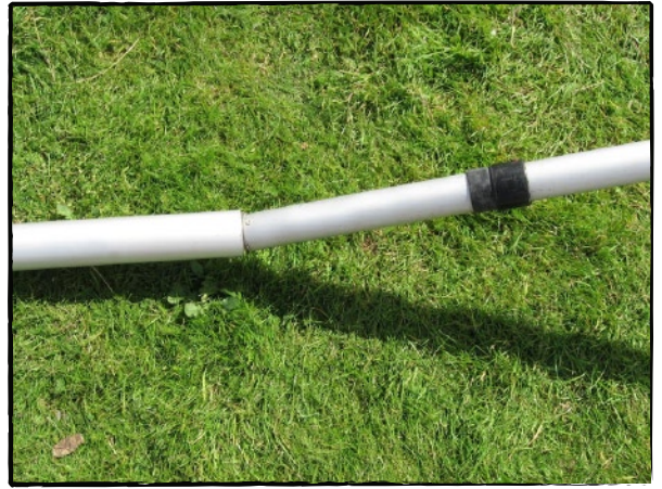
Photo 4, Assemble the two mast halves
