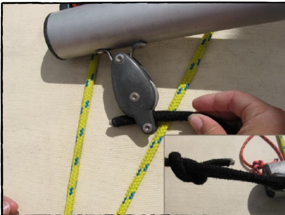
Photo 31, First block and bowline
