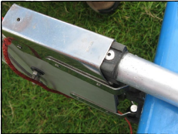
Photo 38, Insert the tiller
